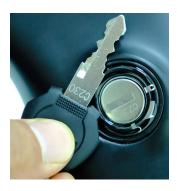
Insert the key to the lock ,rotate to right,the battery will drop till a protection device in the battery case works ,then press the safety lock lever to release the battery
