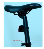
Minimum height of the saddle: move the quick release handle to the OPEN position, then put the saddle post to the lowest place, and when the saddle post cannot enter into the saddle tube of the frame, it is the minimum height of the seat.
