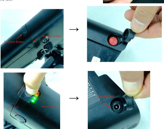
There are three main function on the battery case. The function button could allow riders to press for the battery indicator. The charging port is invisible ,Lift the cover of the other two ,We will find the charging port &the ON/OFF button. Recommend turning to I if not use for a long time
