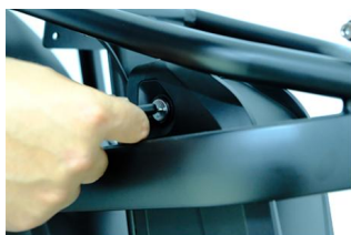
Battery 2: Rotate the key to right, Lift the battery up with the other hand
