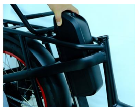
Battery 2: Rotate the key to right, Lift the battery up with the other hand
