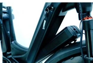
Battery 1: Rotate the key to right, open the safety lock, the battery released
