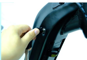
Battery 1: Rotate the key to right, open the safety lock, the battery released
