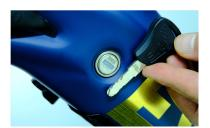
Insert the key to the lock ,rotate to right,the battery will drop till a protection device in the battery case works ,then push the safety lock lever to release the battery
