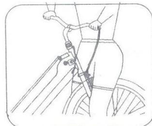
Some models have a light/power meter console that attaches to the handlebar. Attach this with the plastic brackets and screws provided.
