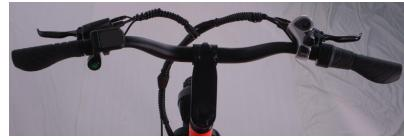
Your handlebars have two main parts--the bar itself and the adjustable stem. If your bar has been removed for shipping, position the bar in the center of the stem and check, to be sure that your grips are in the right place and the angle of the bar is comfortable. Tighten the screws clamp to hold the bar in place, ensuring all brake cables are clear.
