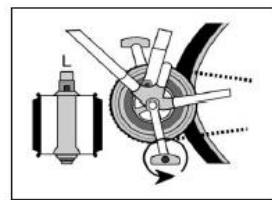
(2). The left pedal attaches to the other arm and has a left-hand (counter clockwise) thread.
